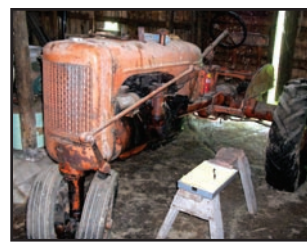
"C" Allis Chalmers hidden barn treasure. Story is it may have been rebuilt and then parked, as it wasn't needed. Has the pulley mounted on rear differential to run accessories, used to run a saw rig.
